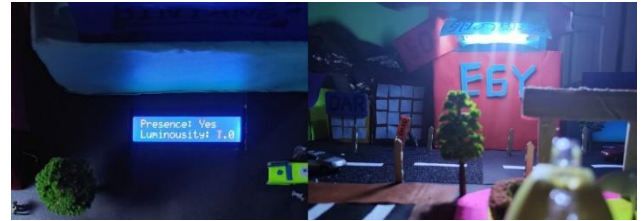
Fig. 18. Testing using the LDR = 1 and PIR = 1 condition tool
