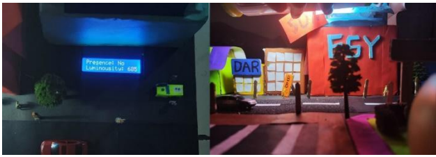
Fig. 8. Testing using the LDR = 685 and PIR = 0 condition tool
