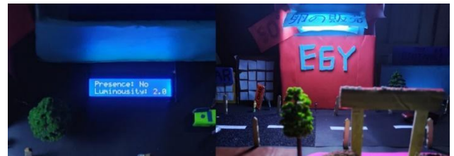
Fig. 20. Testing using the LDR = 2 and PIR = 0 condition tool
