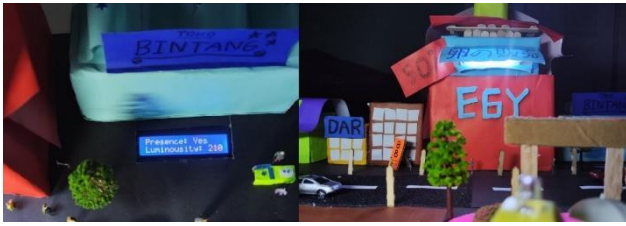
Fig. 14. Testing using the LDR = 210 and PIR = 1 condition tool
