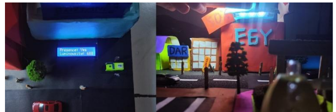
Fig. 6. Testing using the LDR = 688 and PIR = 1 condition tool
