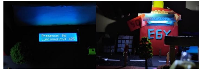
Fig. 12. Testing using the LDR = 423 and PIR = 0 condition tool
