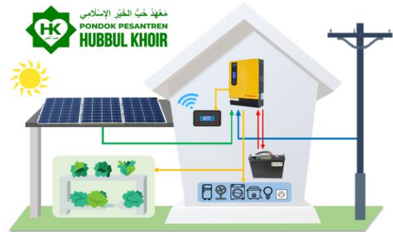
Fig. 5 Solar Power Plant and Monitoring System
