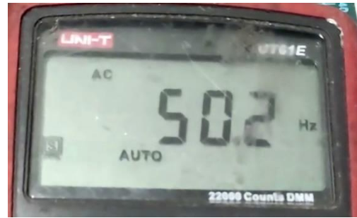
Figure 12. Output frequency measured by multimeter
