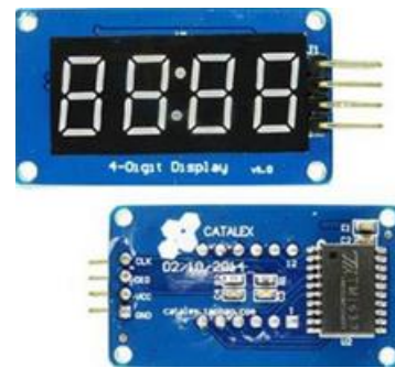
Figure 4. LED TM1637 Display [3]
