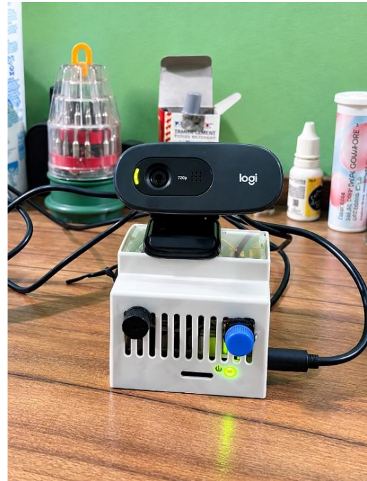
Fig. 2. Hardware prototype of the driver drowsiness detection system.
