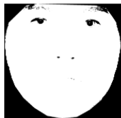
a. Image Otsu threshold result NIR distance 1 meter
