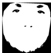
Fig. 7. Otsu threshold result of the image NIR dataset Tuft.
