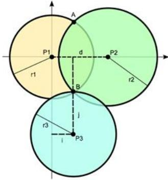
Fig. 2. Illustration of Position Estimation with Trilateration.
