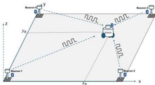
Fig. 1. Illustration of Localization System Based on BLE Beacon.
