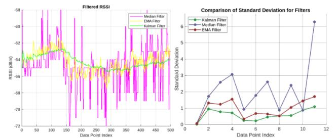
Fig. 4. (a) Filtering Results, (b) Graph of Filters Standard Deviation
