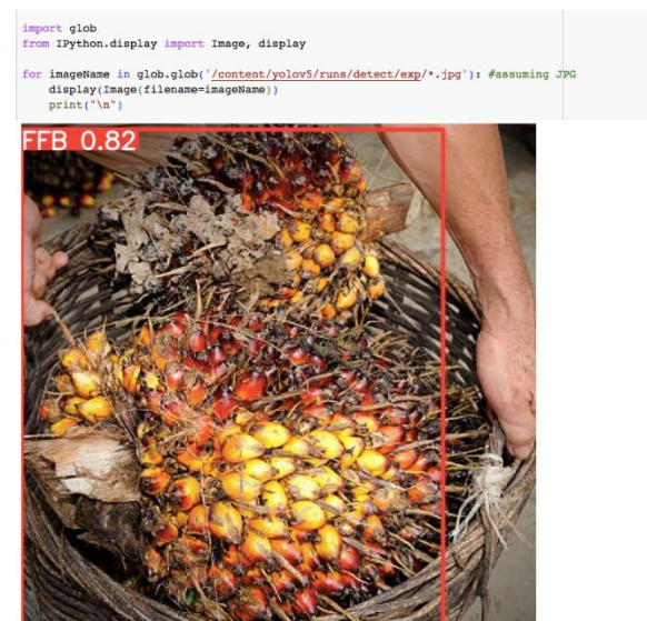
Fig. 6. YOLO-Based Image Detection Output for Oil Palm FFB with Confidence Score Displayed Using Python Script in Google Colab Environment.
