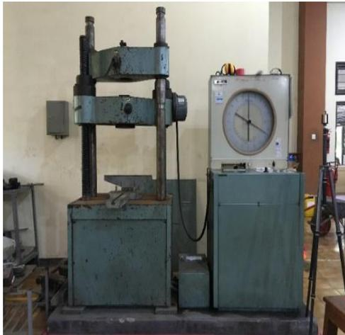
Gambar 3. Mesin Desak / *Universal Testing Machine*
