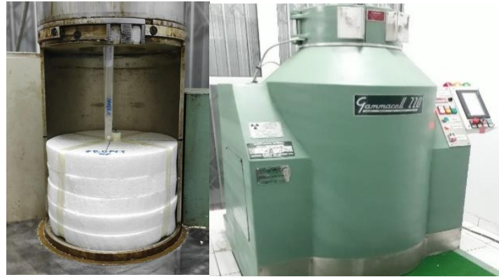
Figure 4. Dose deposit measurement at central position of chamber
