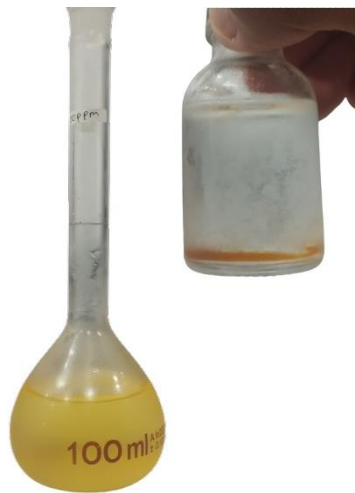
Figure 1. Stock solution of Fe 3+ (left) and iron hydroxide begins to precipitate (right)
