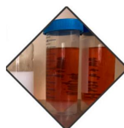
2 g fish scale powder, 20 mL MilliQ water, autoclave, 200°C, 24 hours Figure 9. Carbon Dots Suspension
