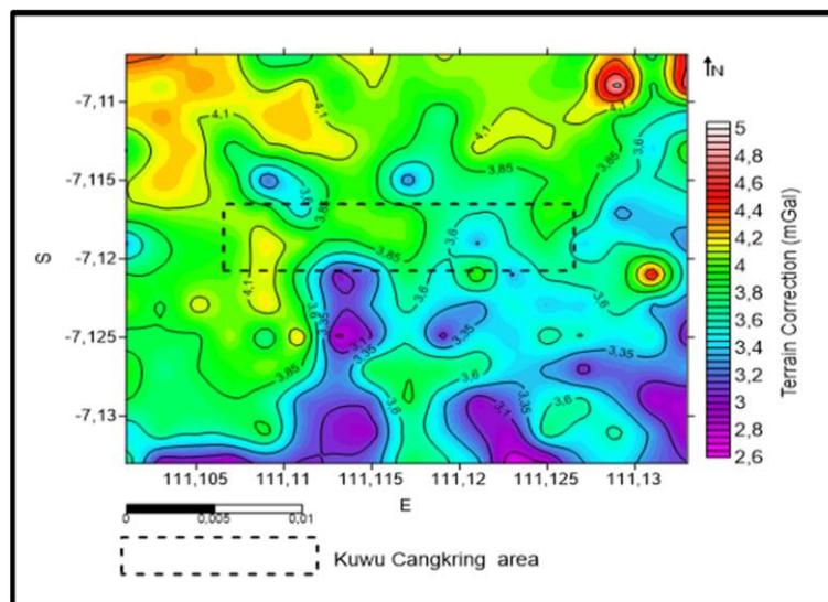
**Figure 5.** Terrain correction map on Bledug Kuwu – Cangkring mud volcano
