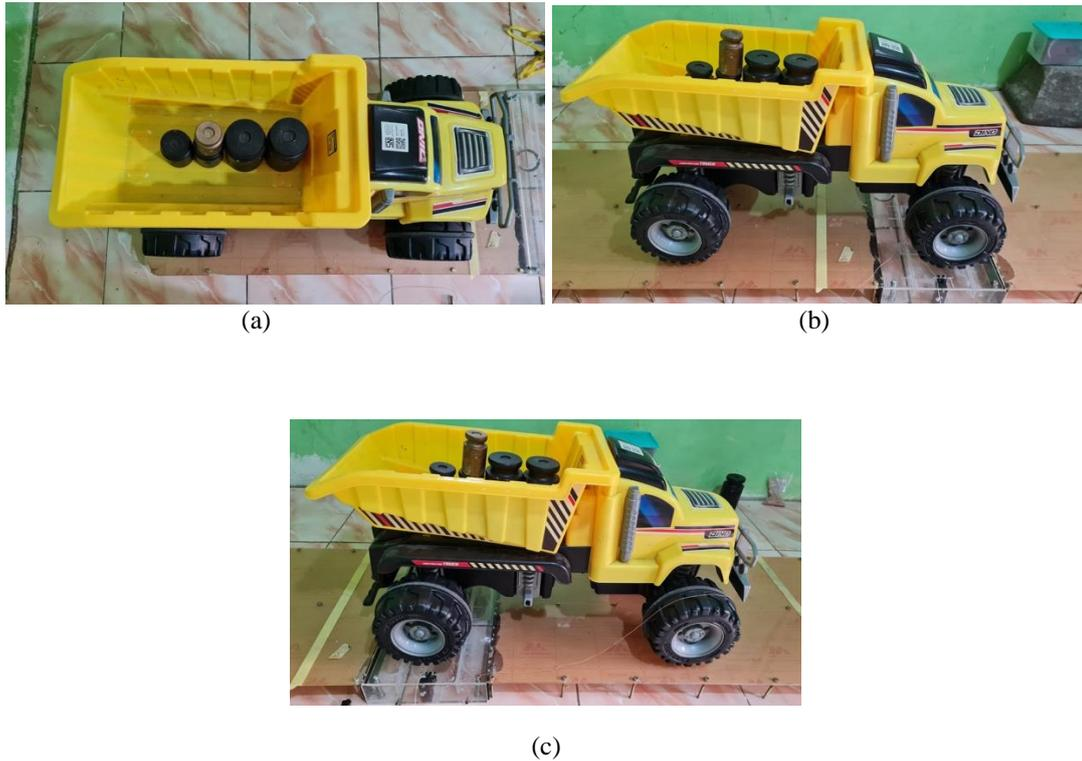
**Figure 5.** Macro bending system testing: (a) Loading on the dummy dump truck; (b) Front wheels; (c) Rear wheels
