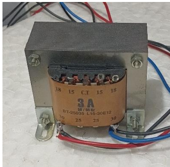
Figure 2. The step-up transformer
