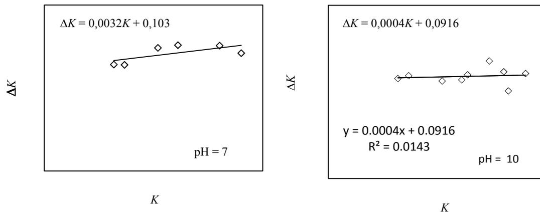
**Figure 2.** Williamson-Hall plots of nanoceria precipitated in (a) pH 7 and (b) pH 10
