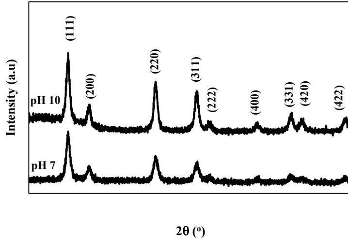
**Figure 1.** X-ray diffraction patterns of nanoceria precipitated in (a) pH 7, (b) pH 10
