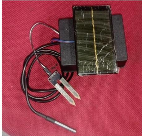
**Figure 1. IoT-based soil monitoring tool**
