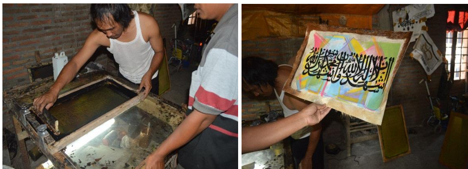
Figure 4. The printing process (left) and check the printed screen printing (right)
