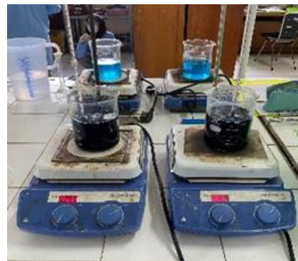
Figure 2. Stirring and heating the solution using a magnetic stirrer
