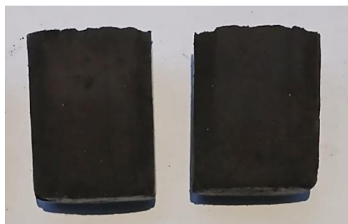
Figure 4. Indigofera tinctoria L. Stems Waste Biobriquettes
