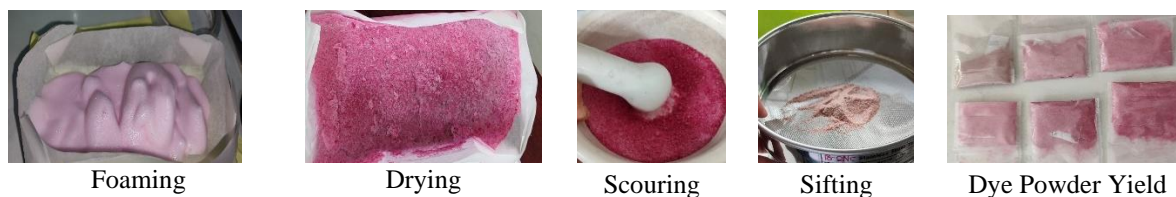
Figure 1. Process for Making Natural Dye Powder
