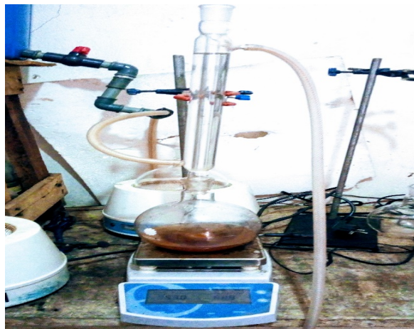
Figure 3. Experimental set-up for biodiesel synthesis
