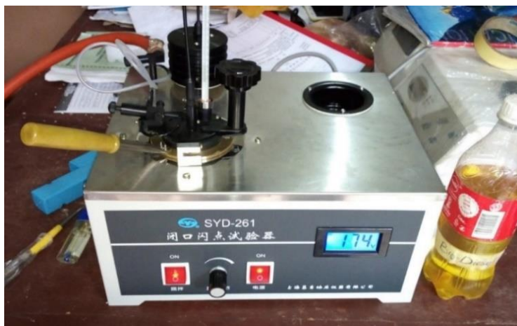
Figure 2. SYD-261 Pensky Martens Closed Cup Flash Point Tester
