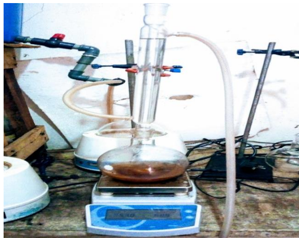
Figure 3. Experimental set-up for biodiesel synthesis
