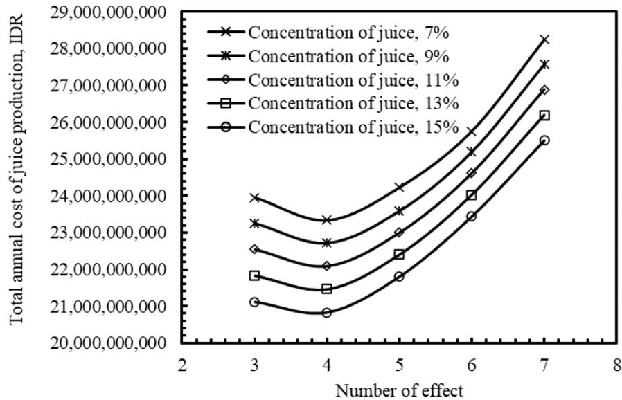
**Figure 5.** Effect of number of effects on total annual juice production cost for various feed juice concentrations at 100°C feed temperature
