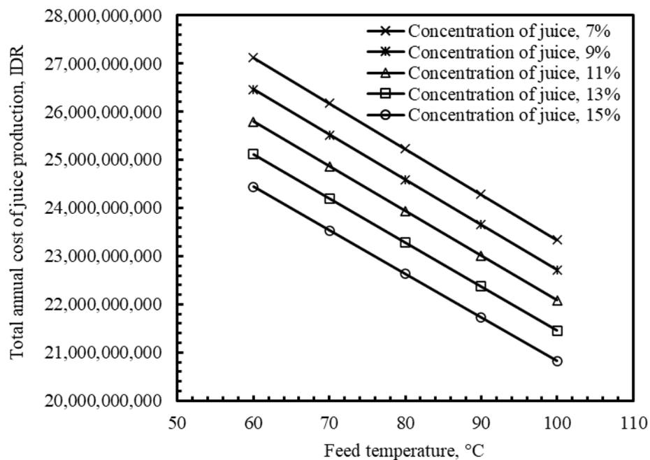
**Figure 6.** The relationship between feed temperature and the total annual juice production cost for various juice concentrations in the feed in a quadruple effect evaporator system.
