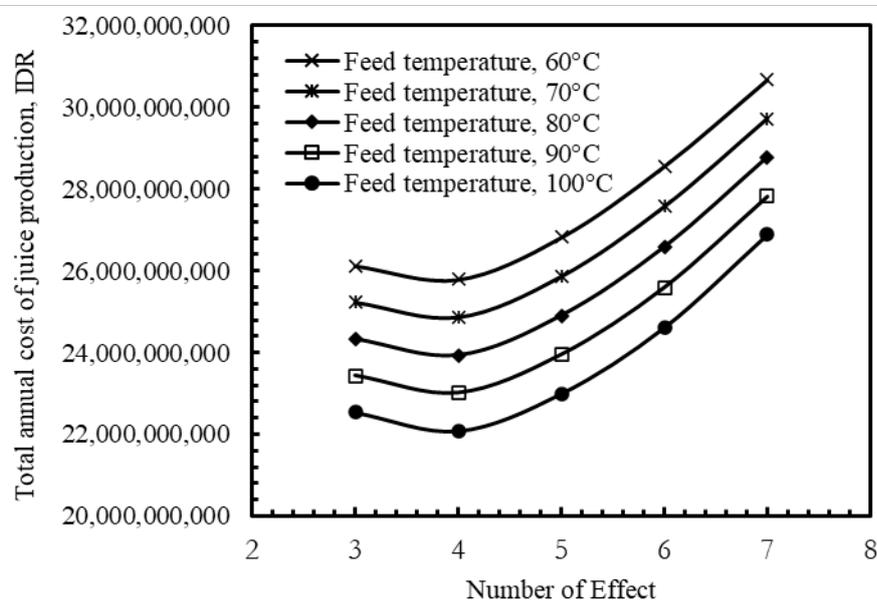
**Figure 4.** Effect of the number of effects on the annual total juice production cost for various feed temperatures at a feed rate of 125,000 kg/h and a feed concentration of 11%.
