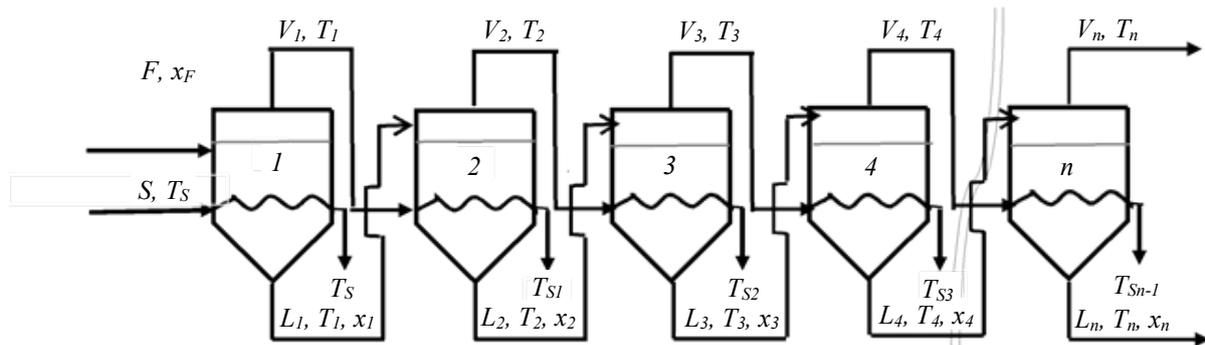
**Figure 2.** Multiple effect evaporator with number of effects n forward feed type
