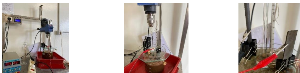
Figure 6. Visual observations of the POME reactor during electro-Fenton treatment at an applied current of 0.25 A: (a) initial reactor condition before treatment, (b) foam and bubble formation following \text{H}_2\text{O}_2 addition, and (c) reactor condition after 5 min of treatment
