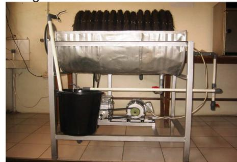
**Gambar 5. Alat RBCs skala laboratorium**
