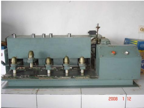
Gambar 7. Crockmeter
