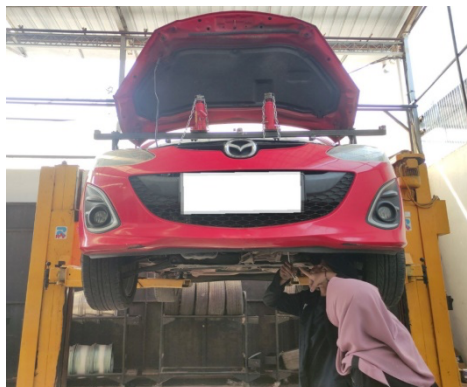
Gambar 2. Implementasi Magnetic Hydraulic Engine Holder
