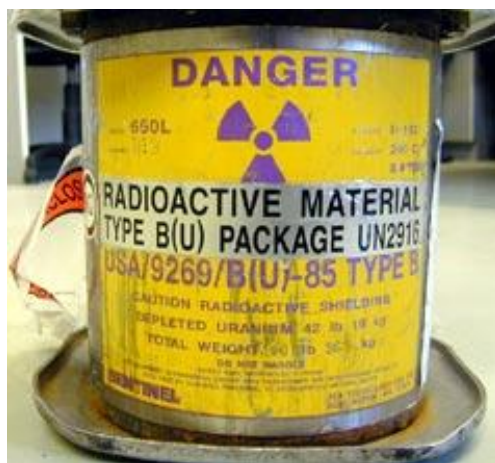
FIG. 7. The example of Type B(U) packages containing radioactive materials .
