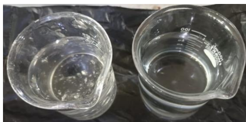
Figure 10. The difference in the solubility test results of (a) oligochitosan and (b) chitosan from tilapia scales.
