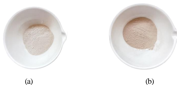
Figure 1. E. guineensis starch powder (a) before and (b) after acid-hydrolyzed modification.
