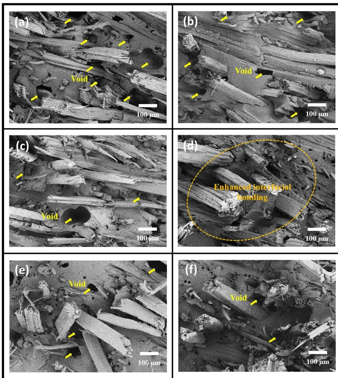
**Figure 3.** SEM micrographs of the tensile fracture surface of composites reinforced with (a) 10% unmodified fiber, (b) 10% modified fiber, (c) 40% unmodified fiber, (d) 40% modified fiber, and (e) 50% unmodified fiber, and (f) 50% modified fiber.
