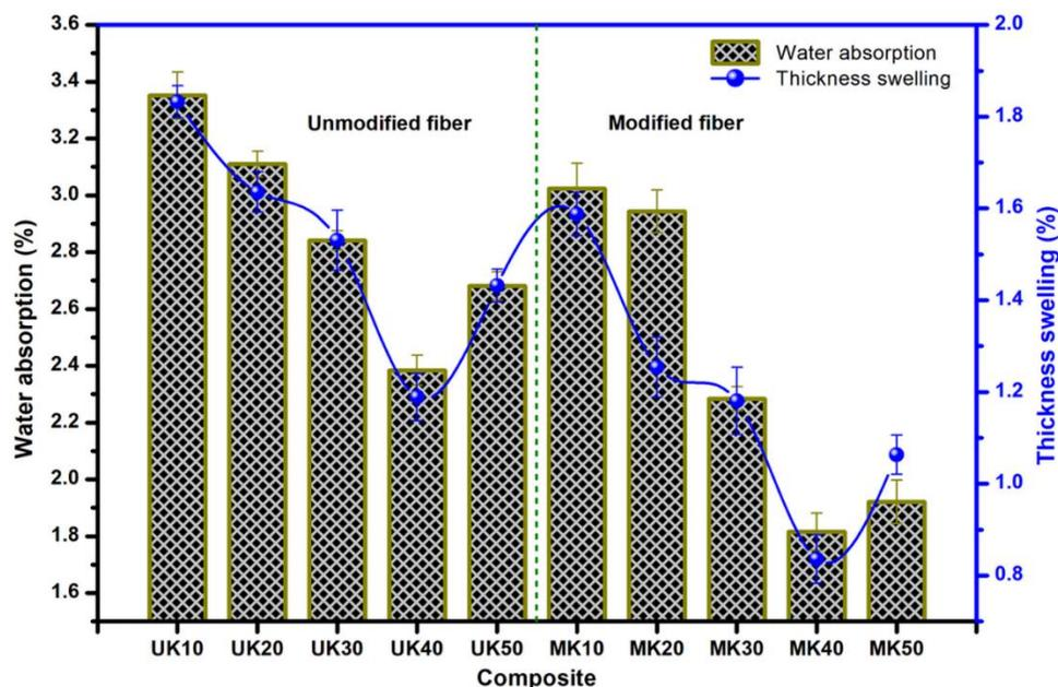
**Figure 1.** Water absorption and thickness swelling of composites reinforced by unmodified and modified kenaf fiber loadings.
