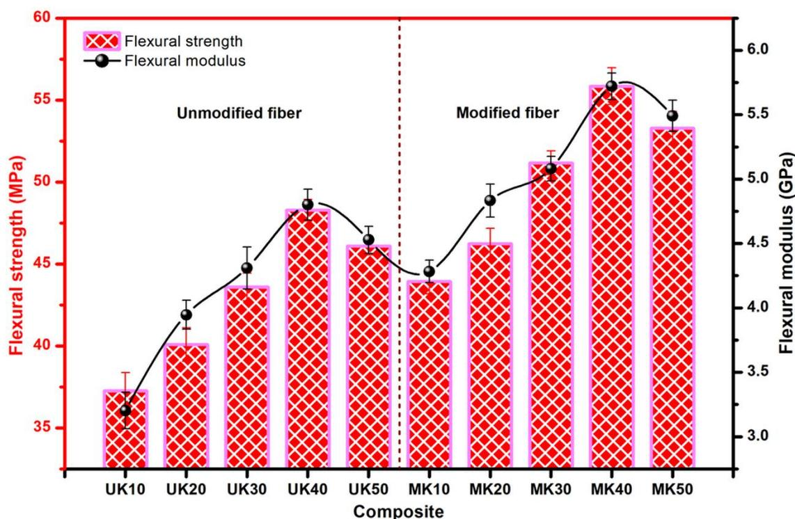
**Figure 4.** Flexural strength and modulus of unmodified and modified kenaf fibers reinforced composites at different fiber loadings.
