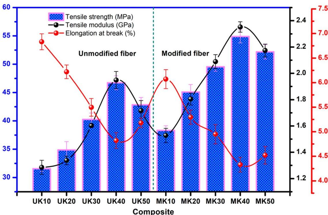
**Figure 2.** Tensile strength, tensile modulus, and elongation at break of unmodified and modified kenaf fibers reinforced composites at different fiber loadings.
