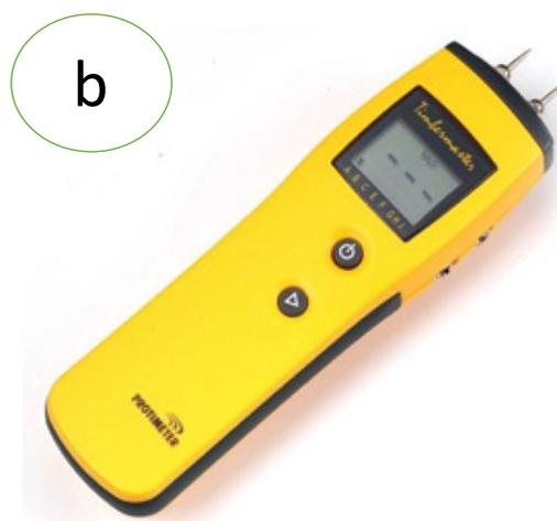
Gambar 6. Alat deteksi kelembaban dinding a) Alumunium foil, b) Protimeter
