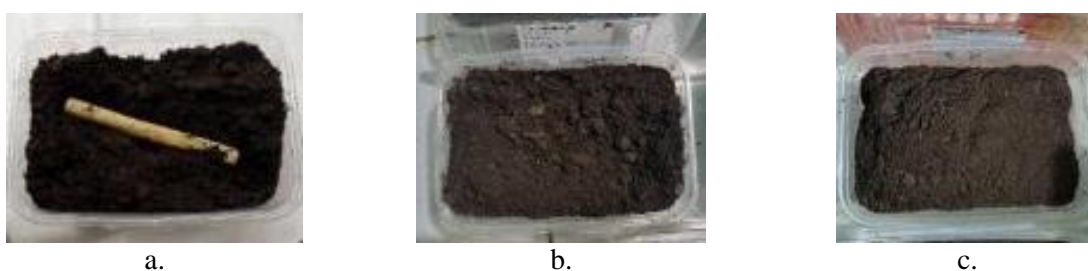
Figure 7. Biodegradability testing process: (a) Day 0, (b) Day 12, (c) Day 15
