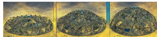
Figure 4. A 1:100 scale generic design was created to investigate the mechanical system and erection technique of the Pantadome. (Photo by Mamoru Kawaguchi)
