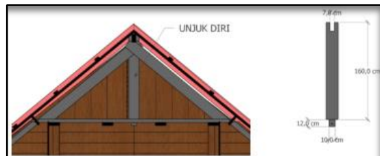
Figure 16. Roof Construction Elements, Unjuk Diri
