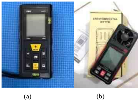
Figure 5. (a) Digital Measuring Device; (b) Digital Anemometer Measuring Device
